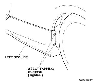
41. Tighten the bracket screw.
