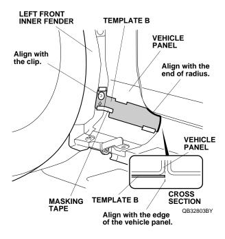
Using a felt-tip pen, mark the vehicle panel in the area shown. Remove template B. Be careful not to damage the template. It is also used to mark the right side of the vehicle.
